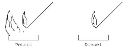
The petrol ignites easily; the diesel only ignites once it has been heated.
