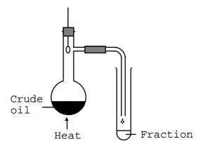
The oil is gradually heated. Fractions, groups of hydrocarbons with boiling points within a given range, are collected.
