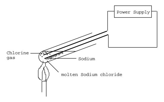
Sodium is obtained at one of the electrodes.
