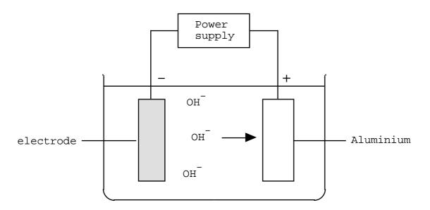
The piece of Aluminium forms the positive electrode. The negative ions are therefore attracted to the positively charged Aluminium and react with it forming Aluminium oxide.
