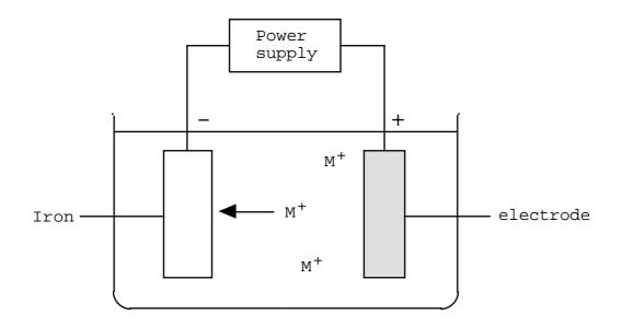
The piece of Iron forms the negative electrode. The positive ions are therefore attracted to the negatively charged Iron, stick to it and form a layer of metal. Tin plating is carried out in this way.
