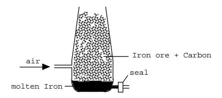
The mixture is heated. Air is forced in at the bottom. The air rushes up through the furnace making a roaring sound. Some of the Carbon burns in the Oxygen. The heat generated raises the temperature of the furnace and the reaction between Iron oxide and Carbon begins:
