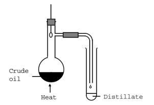
The oil is gradually heated. The small gas molecules boil off first, at low temperatures. We call this the 'gas fraction'. It consists of  $C_1$  to  $C_4$  hydrocarbons e.g. Butane  $C_4H_{10}$  (BP 0 °C). The gas fraction is used to make Calor Gas.
