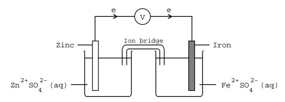
The voltage is so low because the two metals are so close together in the reactivity series. Metals at the top of the series **push** electrons forcibly; metal ions at the bottom of the series **pull in** electrons forcibly. So a combination of a very reactive metal with an ion of a very unreactive metal will give the highest voltage e.g.
