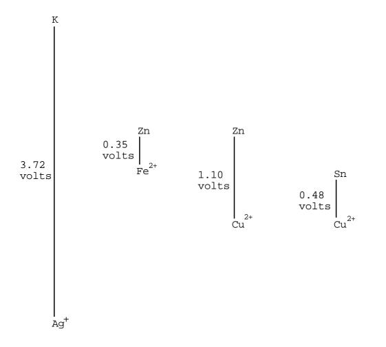
Note that, in a cell, electrons always flow from the most reactive metal to the least reactive metal's ions.
