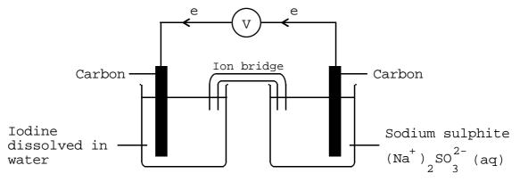
Electrons flow from Sodium sulphite to Iodine (V = 0.37 volts) :
