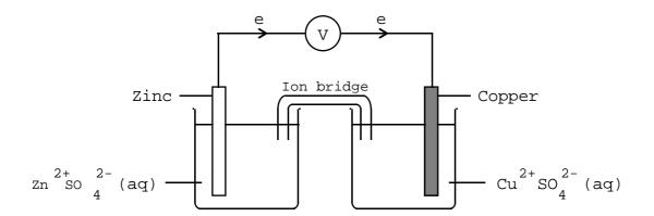
Electrons flow from Zn to  ${\rm Cu}^{2+}$  along the wires and through the voltmeter. This is an electric current.
