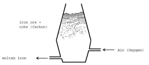
The Carbon monoxide is formed by reaction of Carbon with Oxygen :
