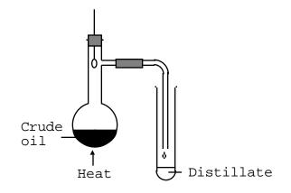
The fractions boil off in the order : gases, petrol etc. The amounts of each fraction depend on the original source of the crude oil. Oil from the Gulf is more viscous and contains more of the heavier fractions than oil from the North Sea.
