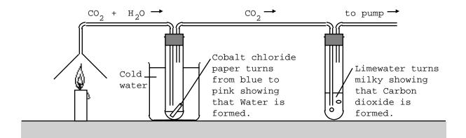
Notice that this experiment shows that hydrocarbons must contain Hydrogen : the Hydrogen in the Water formed can only have come form the hydrocarbon. Similarly the experiment shows that hydrocarbons must contain Carbon : the Carbon in the Carbon dioxide can only have come from the hydrocarbon.
